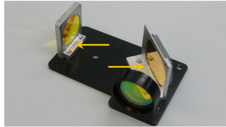
10. Reinstall the Lens Kit in the Focus Carriage.
