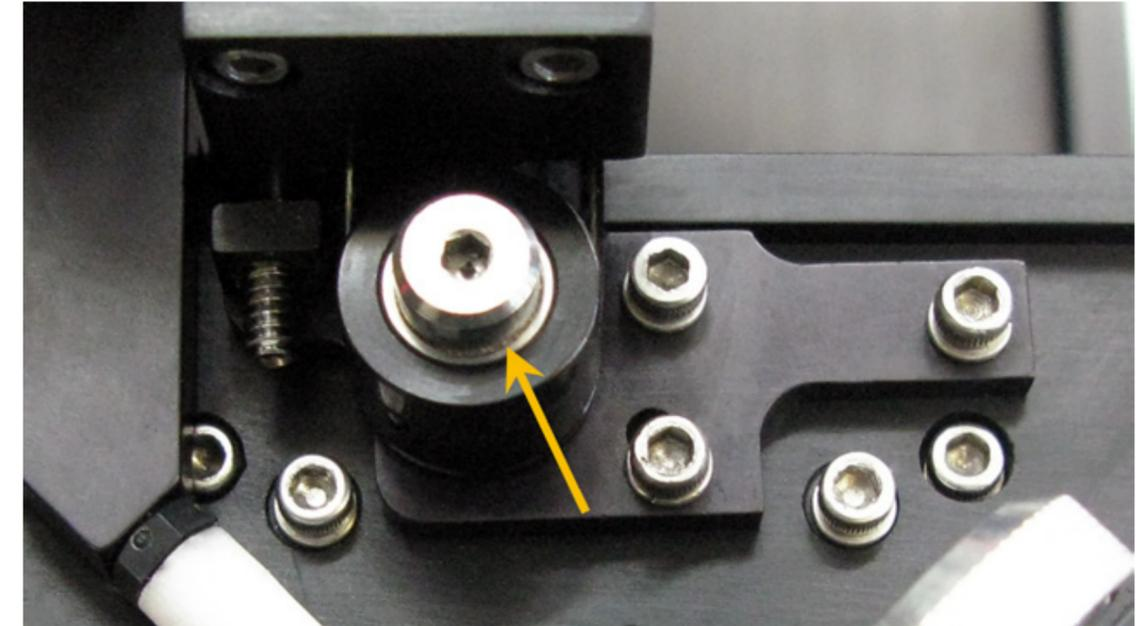
6. When reinstalling the new Idler Pulley insert the pulley at an angle for easier access.
