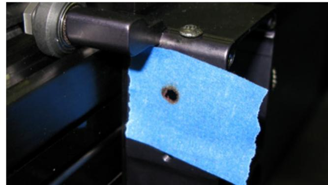
*Correctly Aligned Beam*
