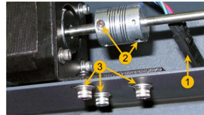
7. Remove the 4 screws securing the motor to the Y-Motor bracket.
