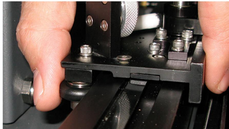
**NOTE:** You should feel an equal turning resistance for each bearing. If one bearing spins freely and the other has a turning resistance, or the turning resistance is unequal, then adjustment is necessary.
