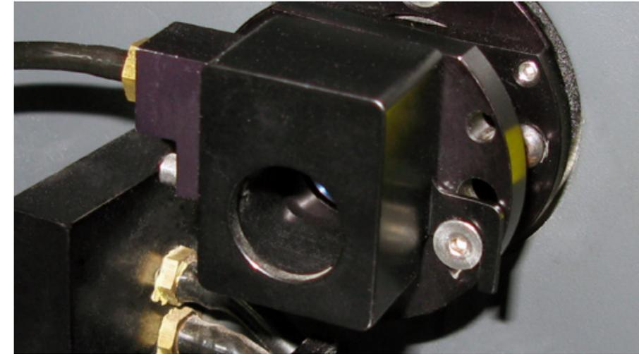
6. Remove the two screws securing the Fitting Block to the Beam Window Protector.
