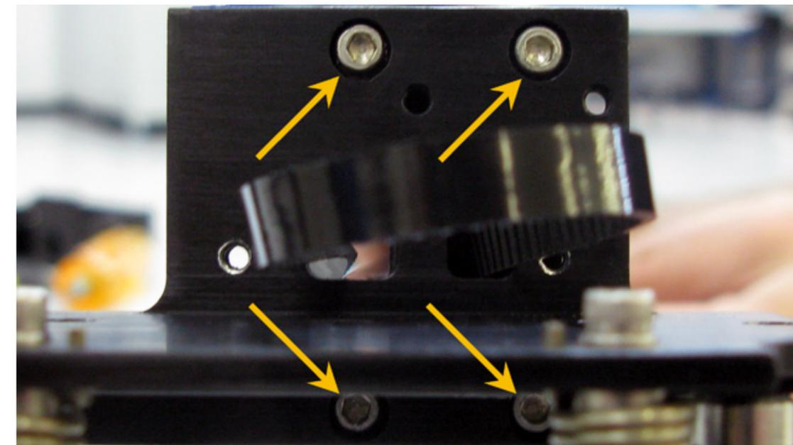
7. Remove the left end support by removing the four screws located on the top (2) and the bottom (2) of the support.
