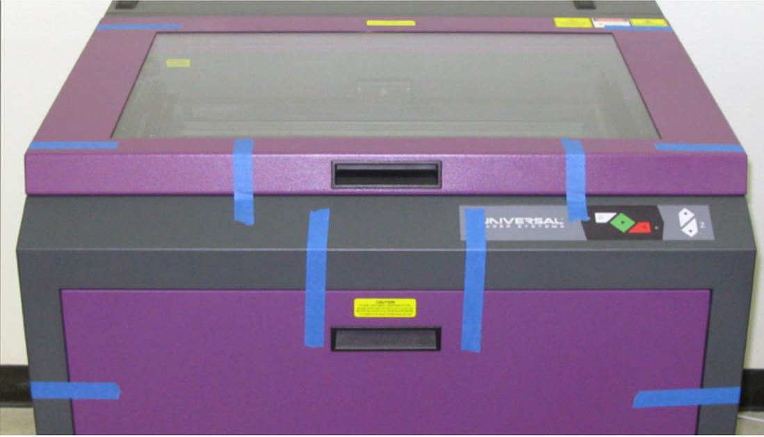
3. Remove the eight screws that attach the cart stand to the laser system, two per leg and four securing the back panel to the bottom of the system, be careful with the washers that contain each screw as these are very important for reassembly.
