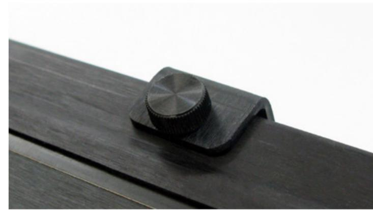
8. Carefully lift the Air Track out of the receiving brackets.
