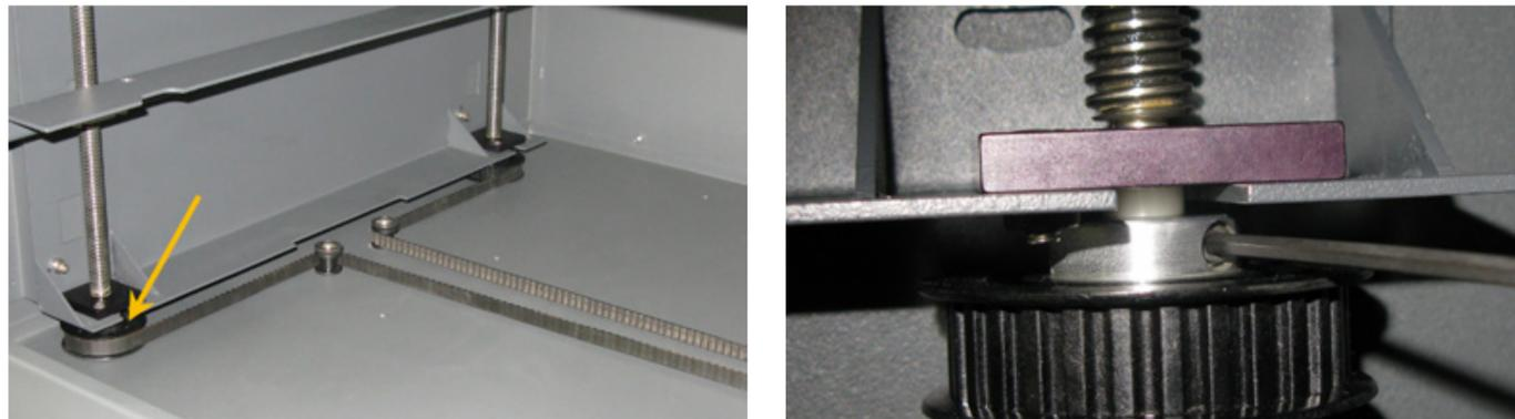
15. Grasp and rotate the threads of the Lead screw and adjust the Table until the focus is the same as for the Upper Left-Hand Corner. Once the left-hand corner is in focus, retighten the Lockdown Screw on the Belt Pulley.
