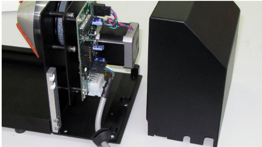
4. Remove the *rotary cone/cup* from the motor end.
