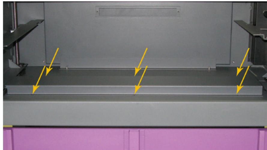
10. With the cover removed, the center portion of the Z belt is exposed. Move the table by pulling on the Z belt (This will move the table much faster than by moving the lead screw).
