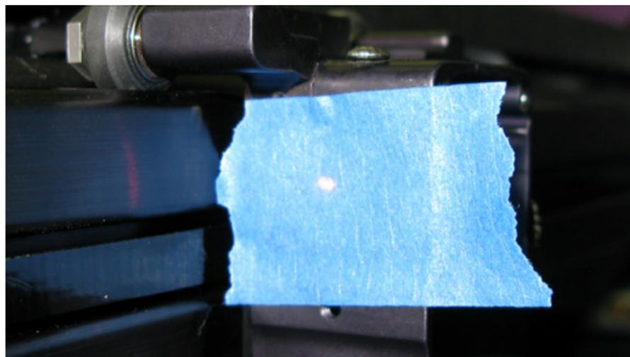
**NOTE:** THE RED DIODE IS ONLY A GUIDE. The red diode may be slightly off-center compared to the burn mark you will make in the following steps, we recommend you make a burn mark for best results.
