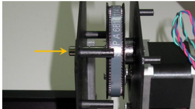
10. Loosen the 4 screws holding the motor in place and shift the motor toward the top of the rear drive bracket. Remove the belt.
