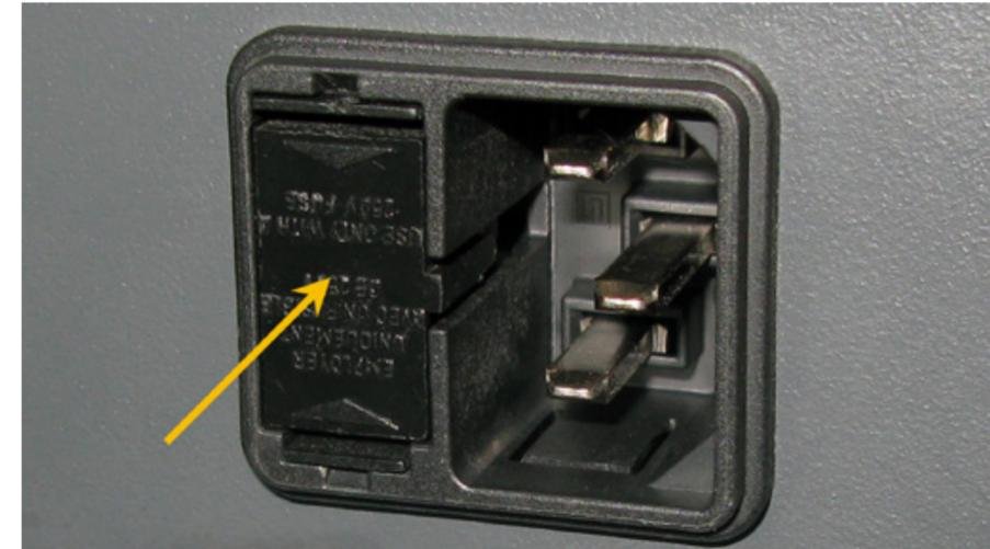
3. Using a small flat head screwdriver remove the fuse drawer.
