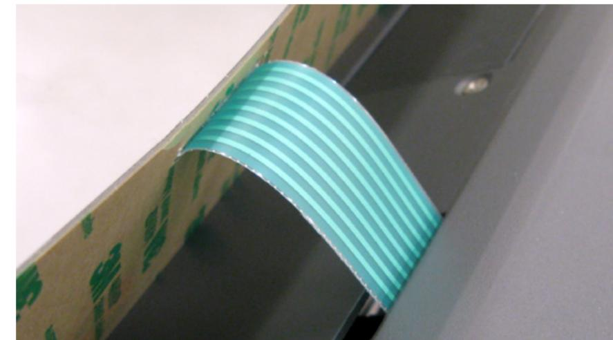
6. Remove the protective backing from the new keypad and slowly apply it to the system, making sure the connector goes to the inside of the system.
