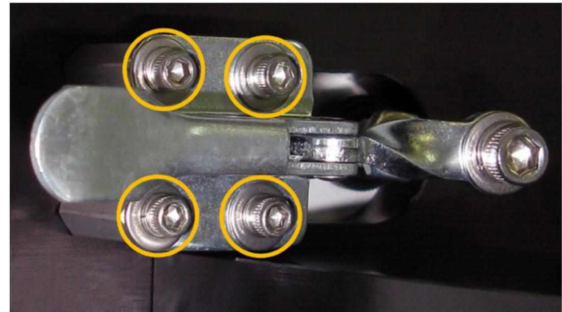
6. Install new toggle clamp with the four screws and washers.
