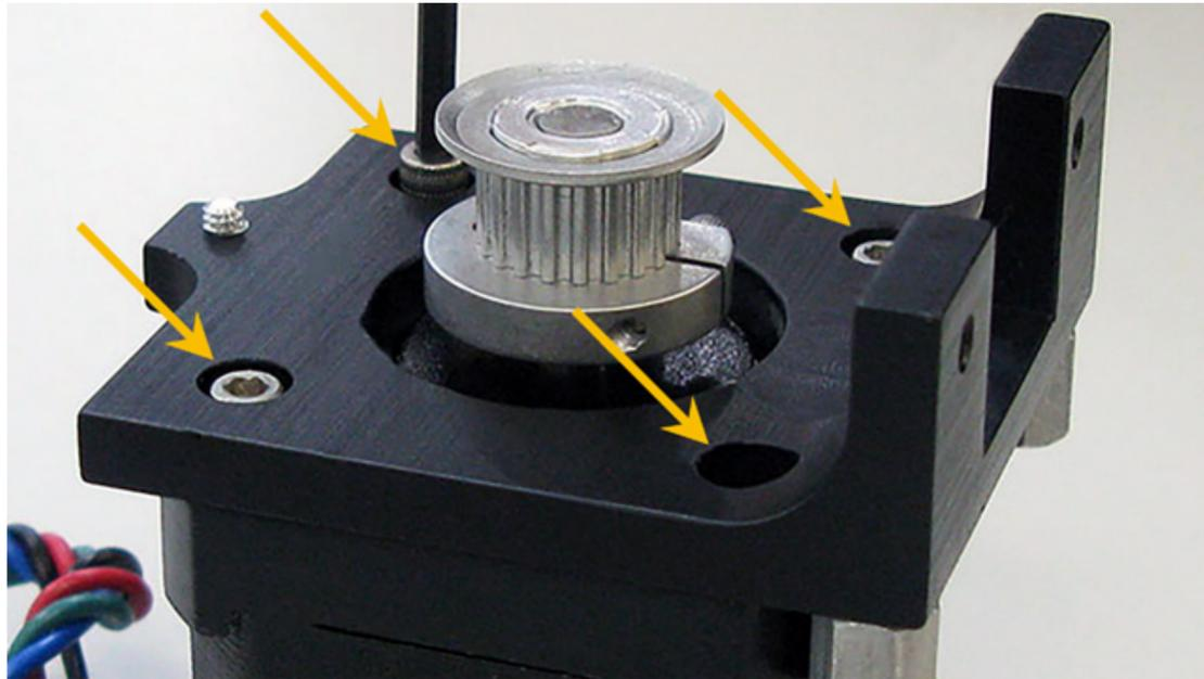
14. Install the drive gear onto the new motor following steps 8 and 9 of X-Axis Drive Gear.
