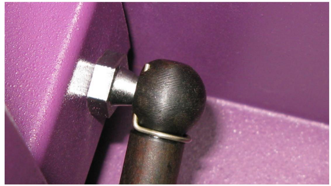
3. Pull the retaining clip down to remove it. Once the retaining clip has been removed the hydraulic pressure cylinder can be removed by pulling outward from the door/system.
