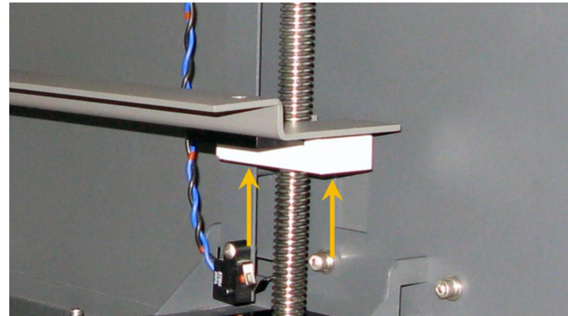
8. Remove the 3 socket head screws, 3 lock washers, and 3 flat washers holding the Right Z-Axis Assembly in place.
