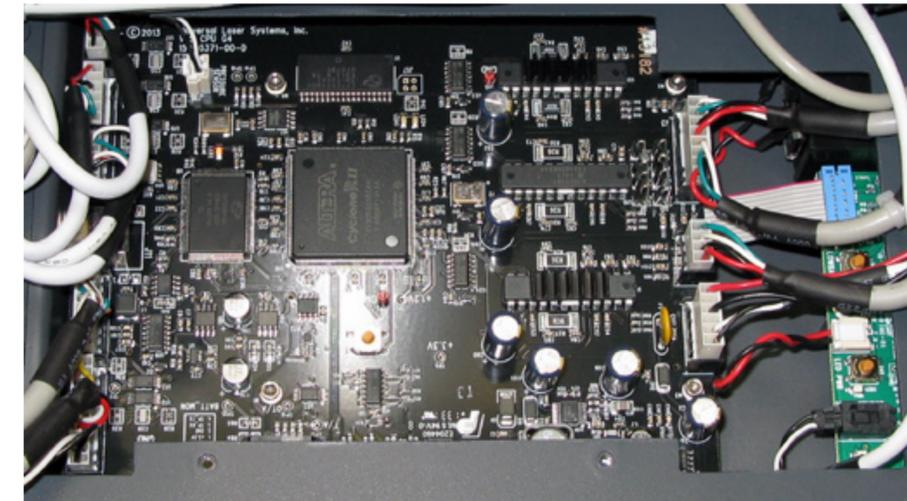
6. Disconnect ALL the wires on the CPU board, including the thermal sensor board wires.
