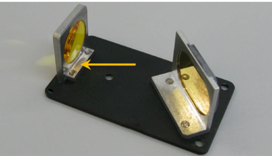
10. Carefully reinstall the Lens Kit using the thumbscrews removed earlier.
