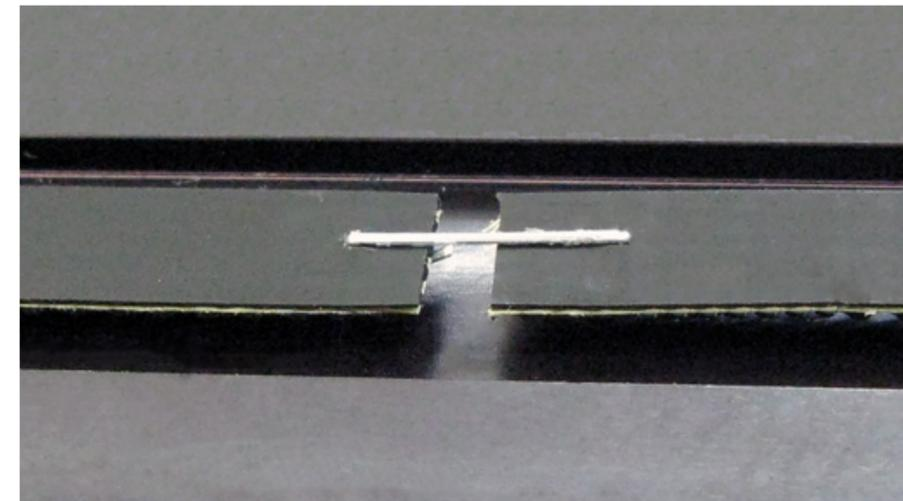
9. Slowly pull the other end of the old belt, allowing the new belt to be pulled through the inside of the X-axis arm. Make sure that you do not twist the belt going through the rail. The teeth of the belt should be facing the inside.
