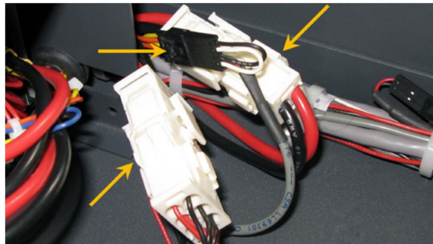
7. Remove the Power Supply Module by carefully lifting up from the Rear Shelf, making sure no cables are pinched in the process.
