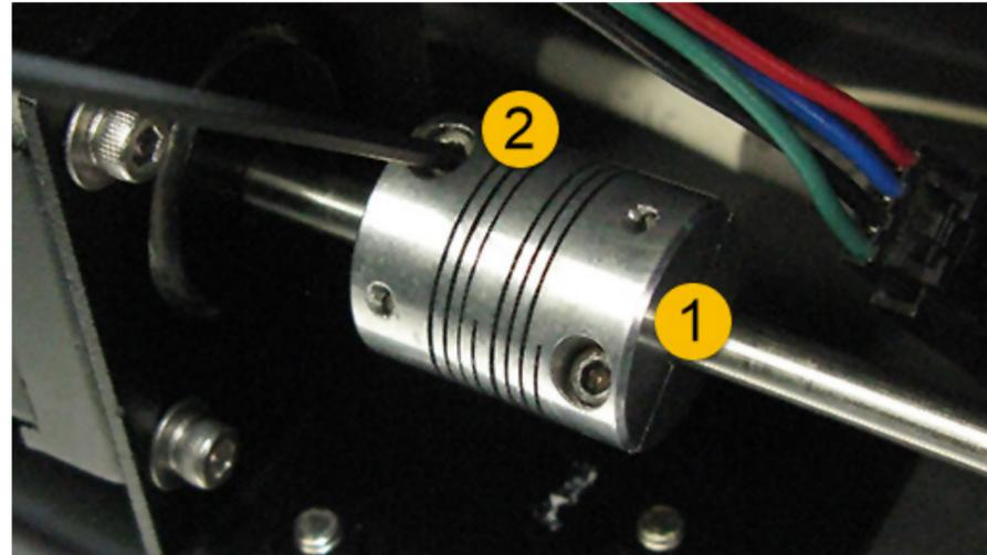
7. Grasp the center of the X-axis arm and pull it forward to contact the shoulder screws. While holding the arm against the two shoulder screws, tighten the screw loosened in the previous step.
