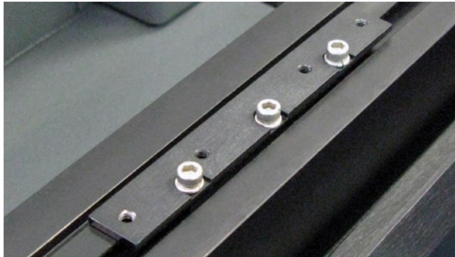
5. After the Y-axis Belt Clamp has been removed staple the new Y-axis Belt to the old belt. Do not overlap the belt and make sure that the teeth are in the same direction.
