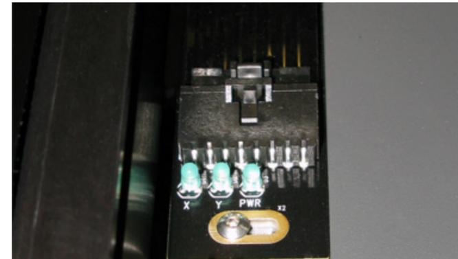
5. Unscrew the 2 screws that hold the board and set side in a safe place.
