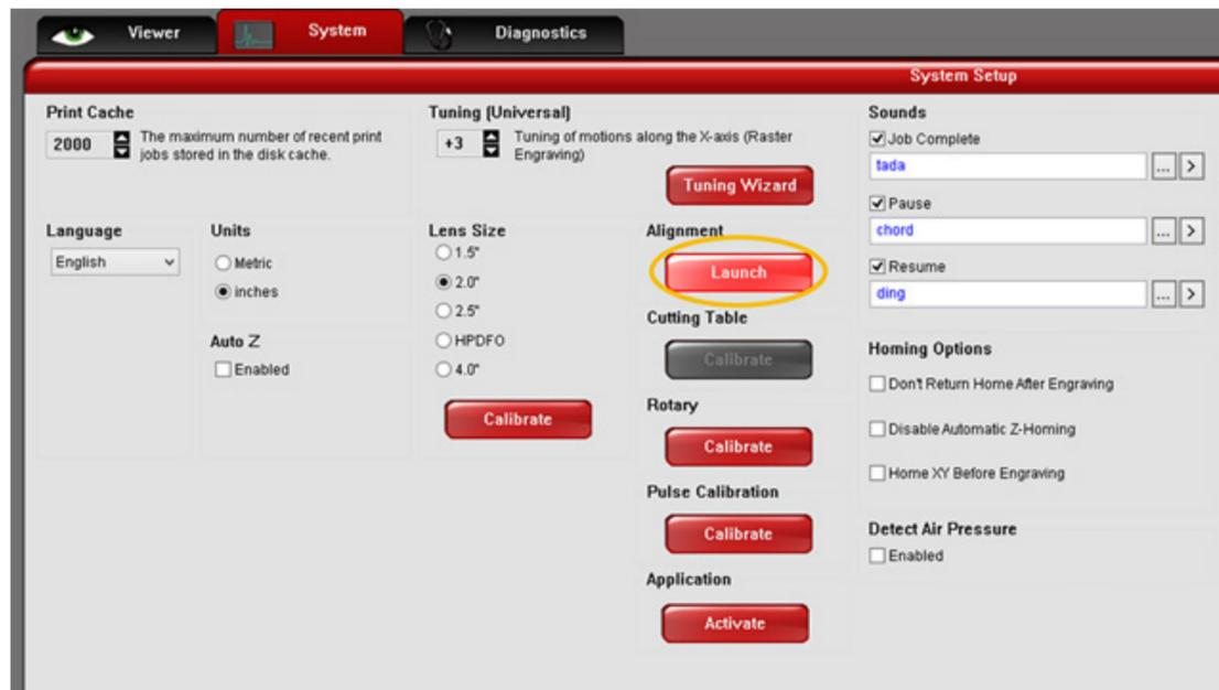
13. On the Alignment Mode Window, click on the Top Left button to move the carriage to the table position closest to the beam window.
