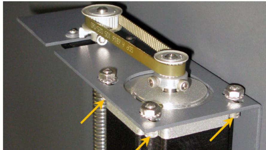
6. With the screws loose, slide the motor toward the lead screw. This will free the small drive belt. Remove the small Z-Axis belt.
