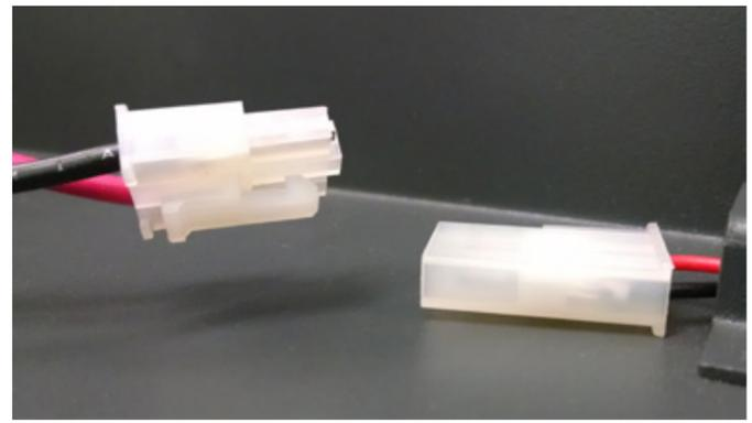
**NOTE:** You may need to temporarily remove the cable tie to gain access to this connection.
