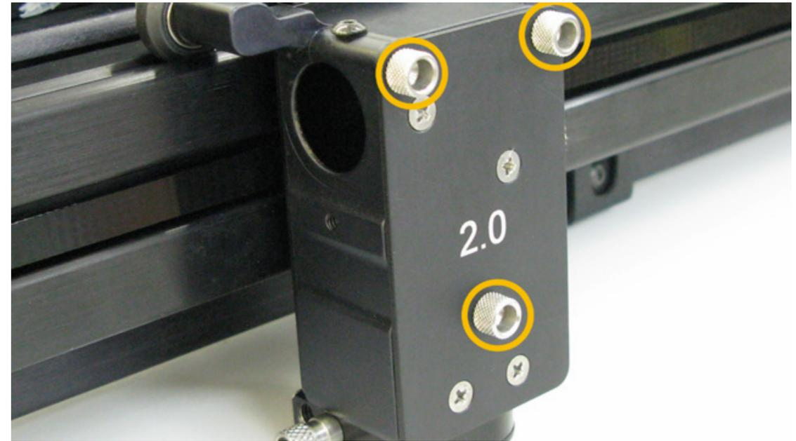
5. Slide the Lens Kit out of the Focus Carriage.
