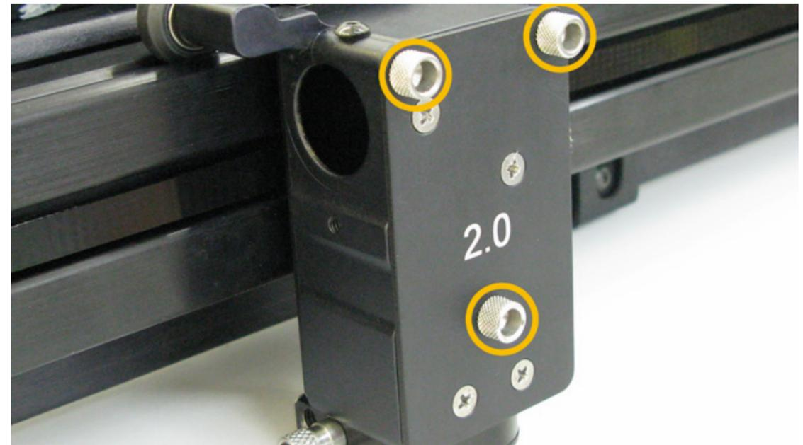
4. Remove the three thumbscrews from the focus carriage. Set them aside in a safe place.
