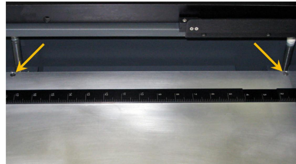
6. Looking underneath the stage locate and remove the two screws and washers holding the right-hand side of the stage to the right table support. Set the screws aside.
