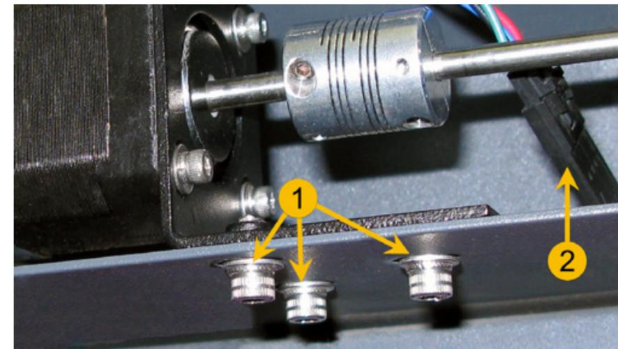
7. Rotate the long shaft with one hand to locate the Y-axis Drive Gear clamp screw (1). Loosen but do not remove the screw.
