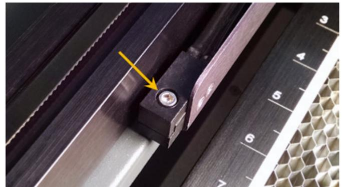
7. Locate and remove the 3 or 4 thumb screws (depending on the size of the system) holding the Air Track to the Air Assist Receiving Brackets.
