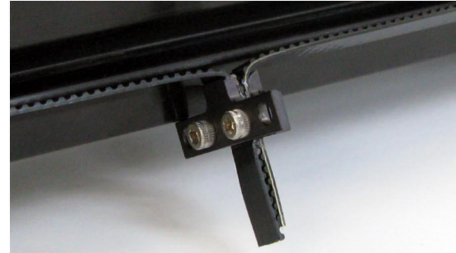
8. Using a stapler, attach one end of the old belt to one end of the new belt. Do not overlap the belt and make sure that the teeth are in the same direction.
