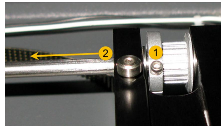
9. Remove the drive gear and replace it with a new one.
