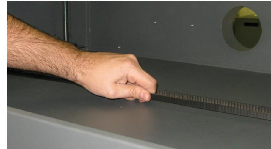
11. Move the table up to the correct height to focus the Upper Left Corner of the system.
