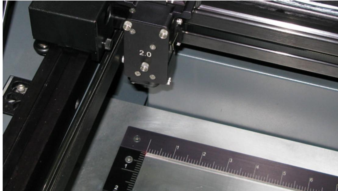
8. If the table is too low it will be necessary to move the right lead screw by hand. Turn the lead screw until the table raises high enough that you can access the long cover plate that covers the middle portion of the Z serpentine belt.
