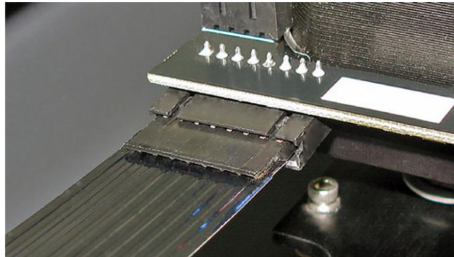
5. The Lower Flex Board is located on the right-hand side near the pressure cylinder. Unplug the other side of the Flex Cable from the Lower Flex Board by pressing on the plastic tab and gently pulling the connector.
