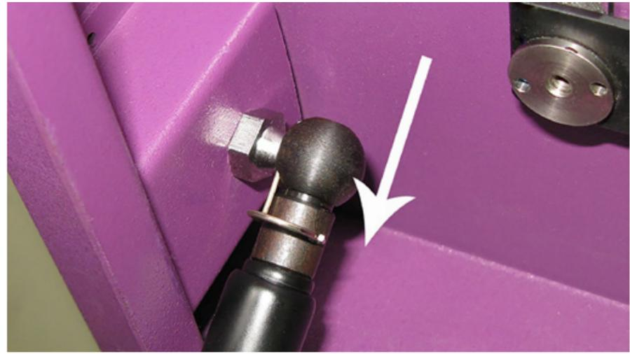
4. Move the hydraulic pressure cylinder out of the way by gently laying it inside the system.
