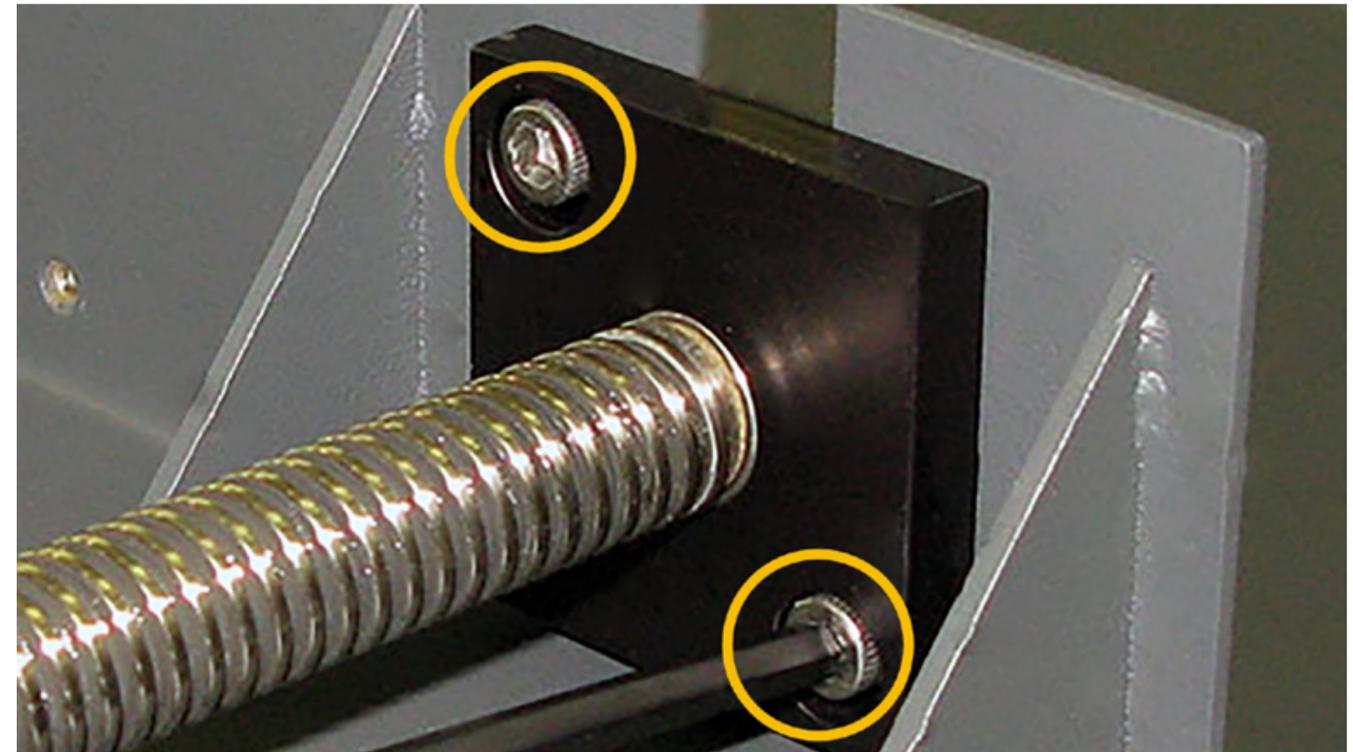
3. Slide the lead screw from the assembly.
