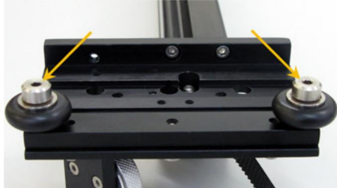
4. To replace the Y-axis Bearings on the right-hand side of the X-axis Arm push the Y Tensioner arms inward (1). Continue pushing the tensioner arm and the Shoulder Screw will be accessible to allow you to replace the Y-axis Bearing (2).
