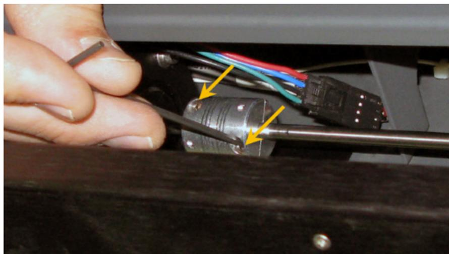
5. Slide the couplers away from the Y-axis Motor.
