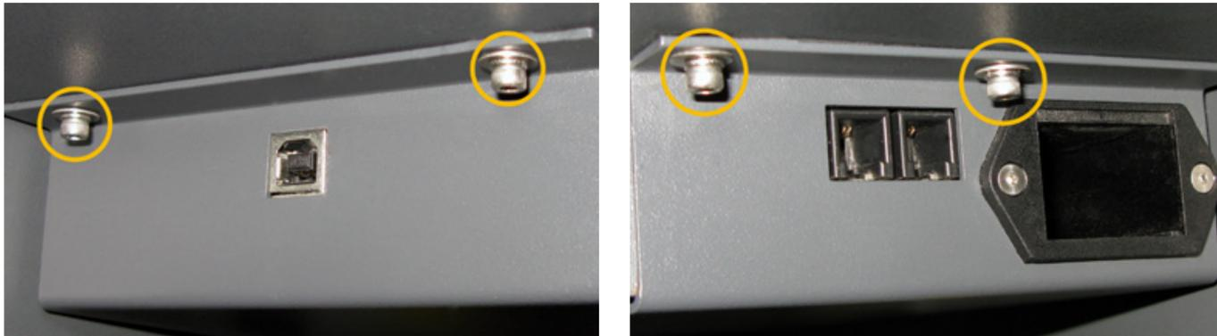
8. Remove the 4 screws holding the CPU in place.
