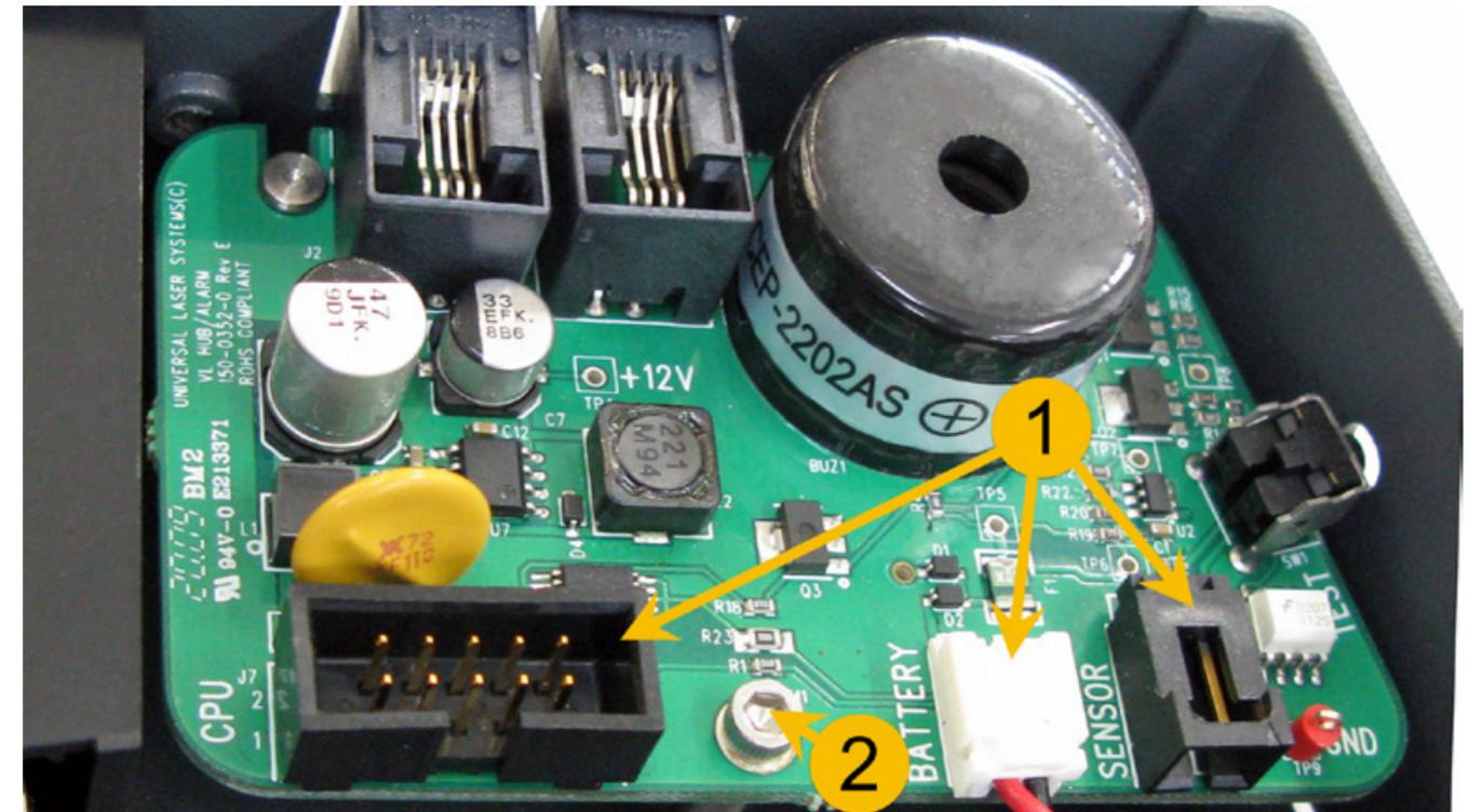
6. Remove the mounting screw (2) from the thermal sensor/com board and slide the board out, being careful not to damage the testing button.
