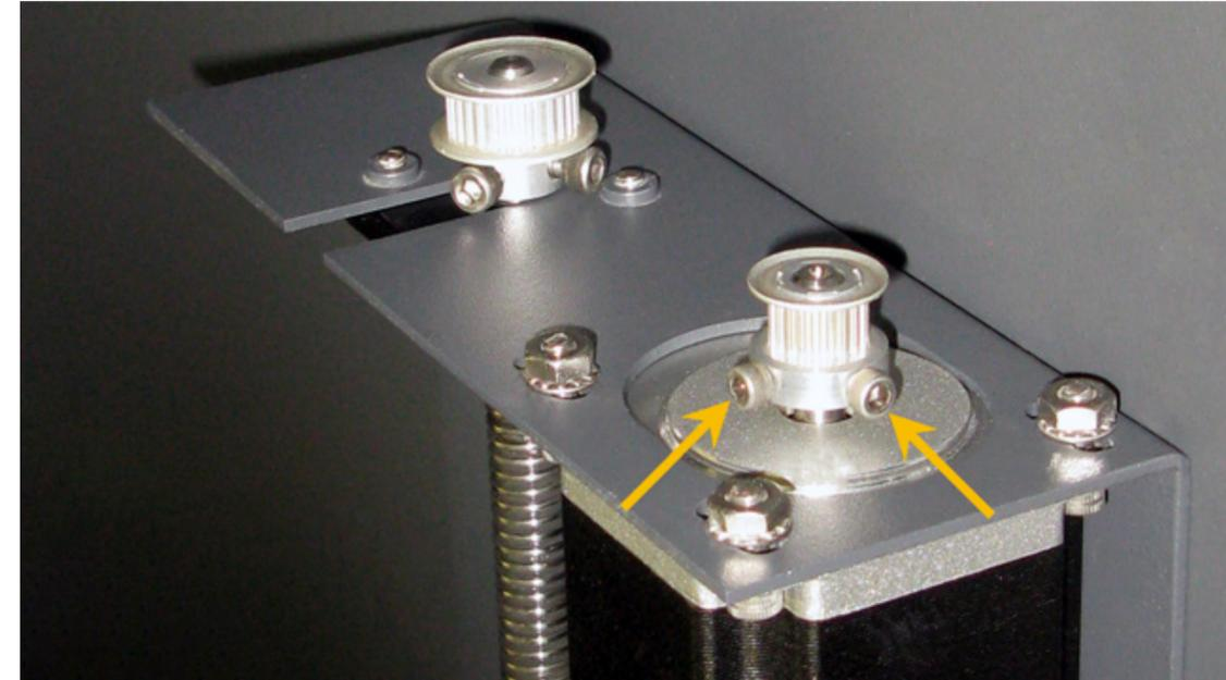
8. Remove the 3 screws loosened in step 5. Remove the motor from the laser system.
