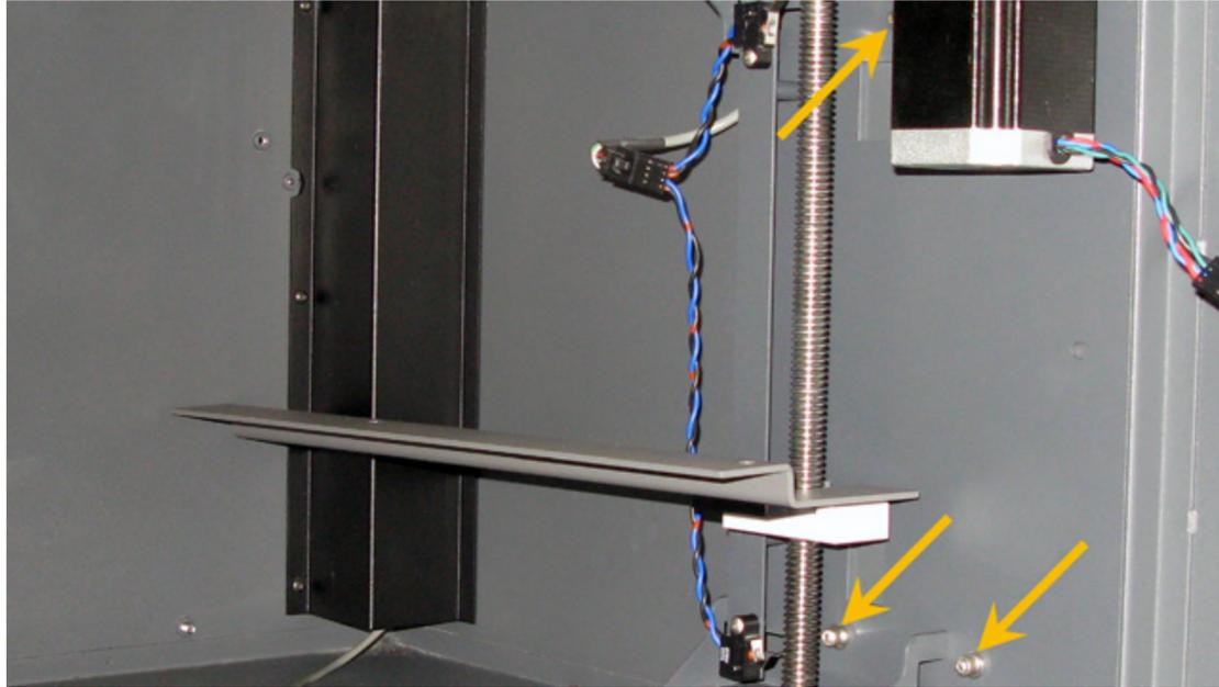
9. Remove the Right Z-Axis assembly from the system.
