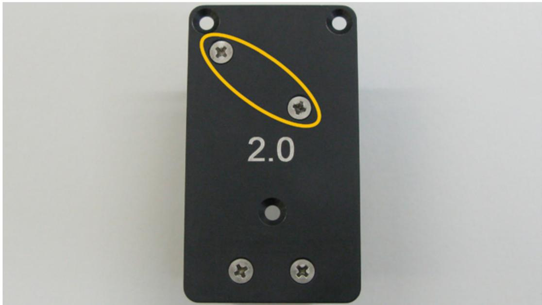
8. Attach the new #3 Mirror to the Front Cover Plate. Leave the Phillips head screws slightly loose.
