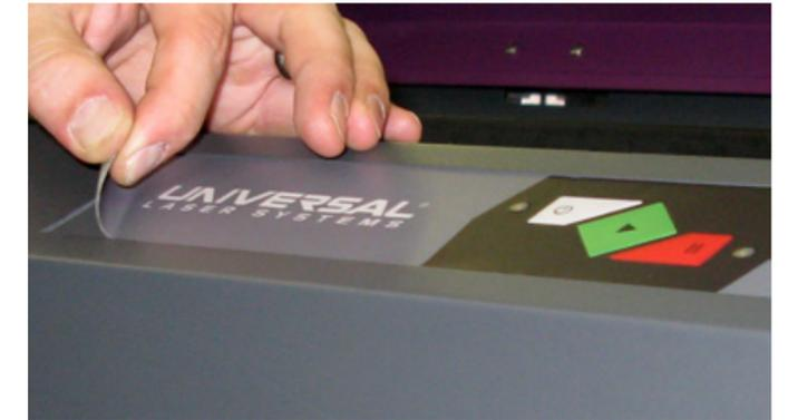
5. Remove the keypad from the front of the machine by slowly peeling it off. Keep in mind that the keypad is an electronic sticker.
