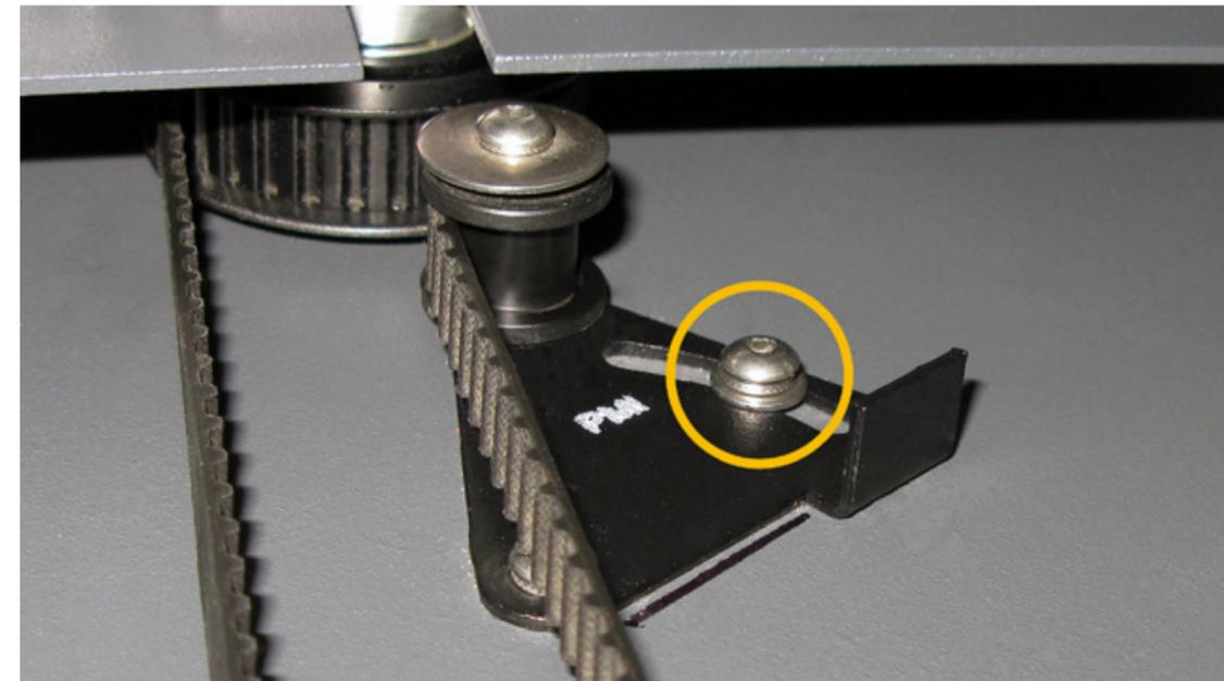
6. Slip the old belt off and slide it under the lead screw pulleys.
