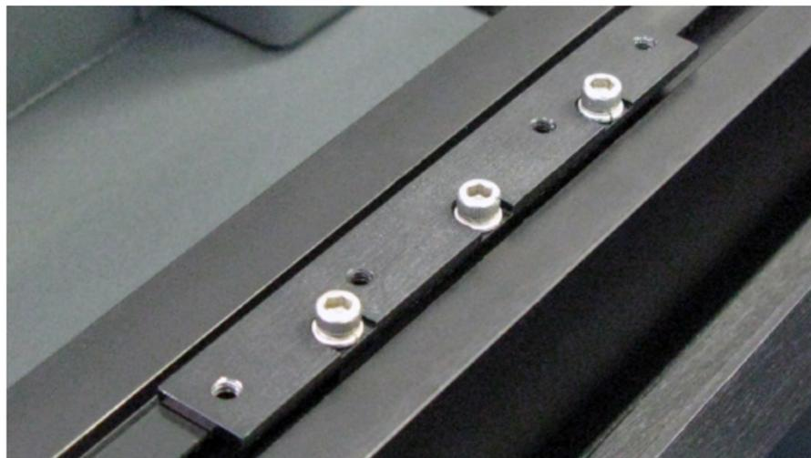
4. Loosen all the Y-axis Coupler screws that are near the Y-axis Motor.
