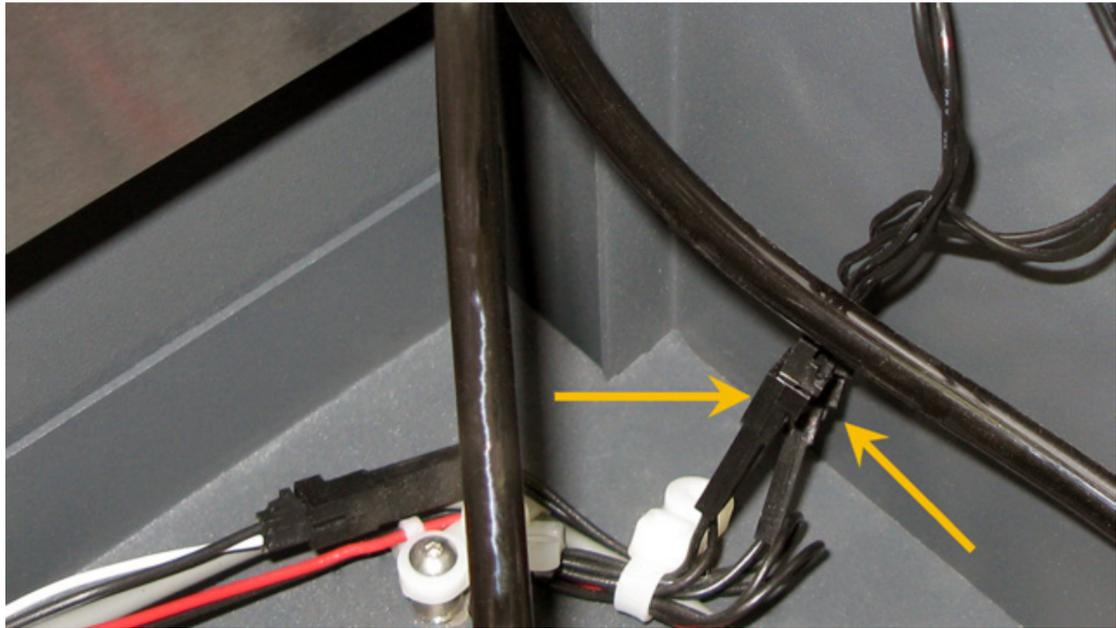
5. Remove the two screws holding the interlocks in position.
