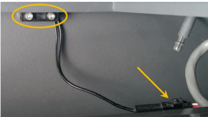
6. Installation is opposite of removal. Ensure the interlock is flush with the frame of the system.
