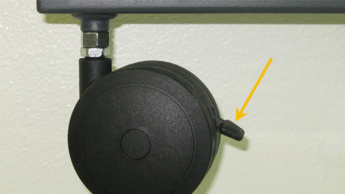
3. Slightly lift the corner of the cart where the caster will be removed.
