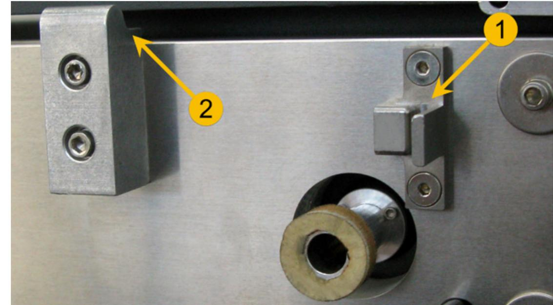
6. From the optics side of the laser (opposite to the connector) have the frame of the laser rest in the center of the alignment fork with the larger tab exposed to the outside.
