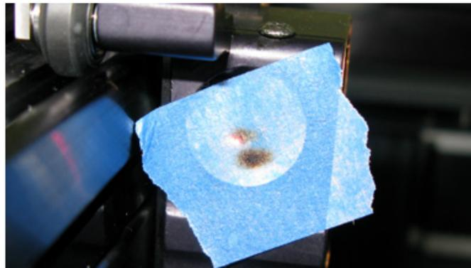
*Incorrectly Alignment Beam*
