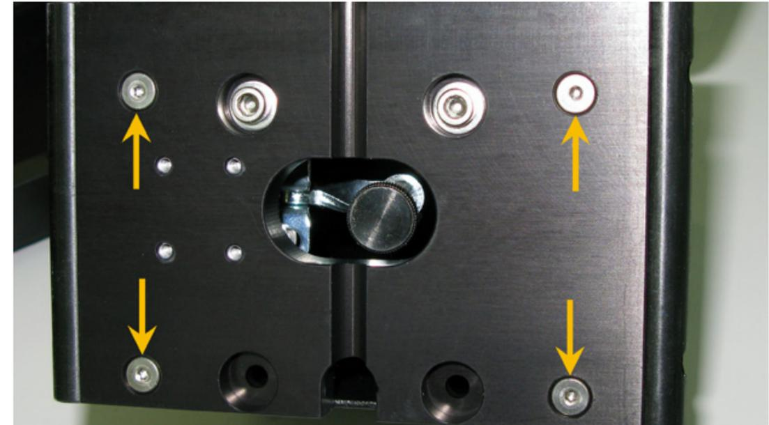
5. Remove the four screws and washers securing the toggle clamp.
