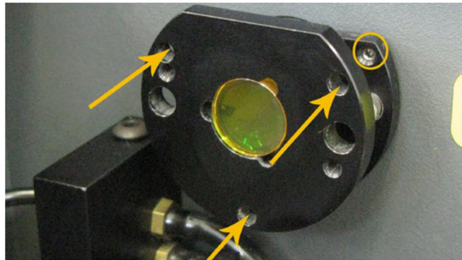
**NOTE:** Access the setscrews through the holes on the front of the collimator.
