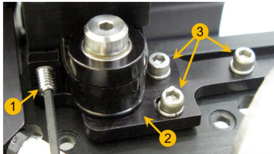
6. Remove the 2 screws located to the right of the Focus Carriage on the belt clamp. Be careful not to lose the washers.
