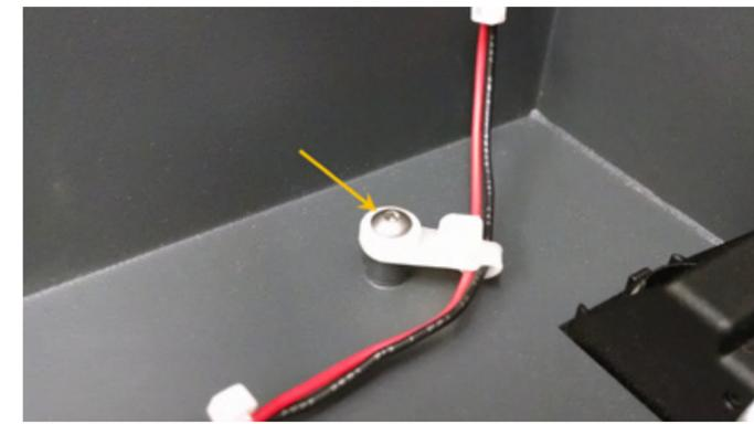
6. Disconnect and remove the power cable. Set the cable aside.
