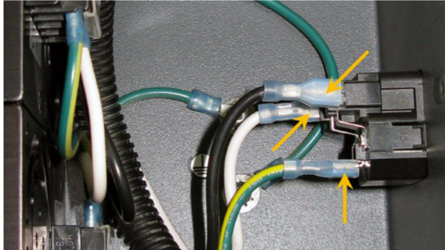
5. Press the tabs on the side of the AC Inlet and push out of the power supply housing.
