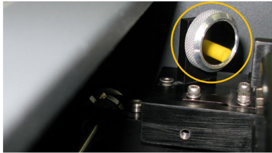
**NOTE:** DO NOT remove the screws behind the mirror. This assembly is spring loaded.
