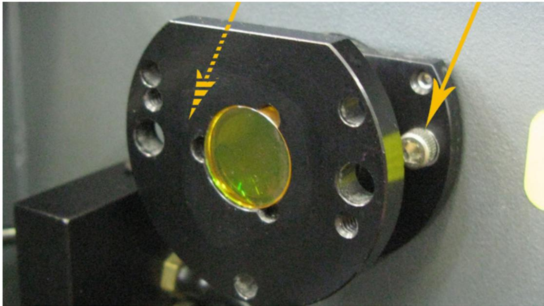
4. Carefully remove the Collimator and place in a safe location.
