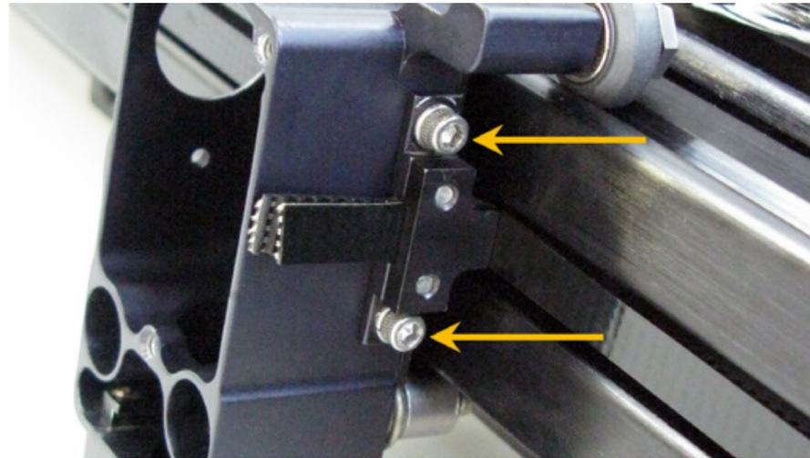
5. If Air Assist is installed, unscrew the two screws that hold the Hook Manifold in place and set the screws aside. DO NOT pull the Air Assist hoses out of the Air Assist Track.
