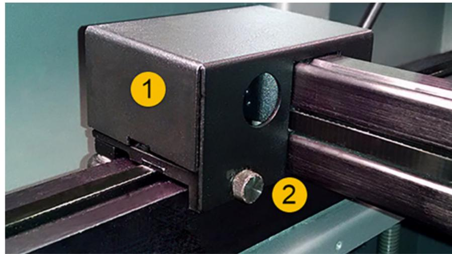
4. Grab hold of the Bezel Mirror Holder and turn it counter-clockwise to remove it. Place it in a safe place.
