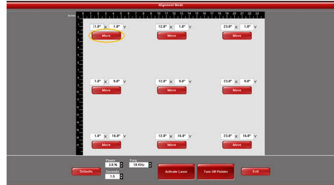
**NOTE:** To create a small burn mark on the tape in the next step, adjust the Power and Seconds settings in the Alignment Mode screen (see picture). Lower power laser systems require higher power settings and higher power laser systems require lower power settings to make the burn mark on the tape.
