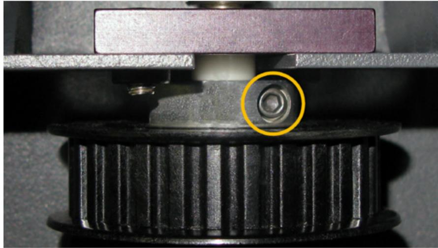
**NOTE:** When removing the bottom pulley be careful as a white spacer may fall off. Remove the spacer and set it aside.
