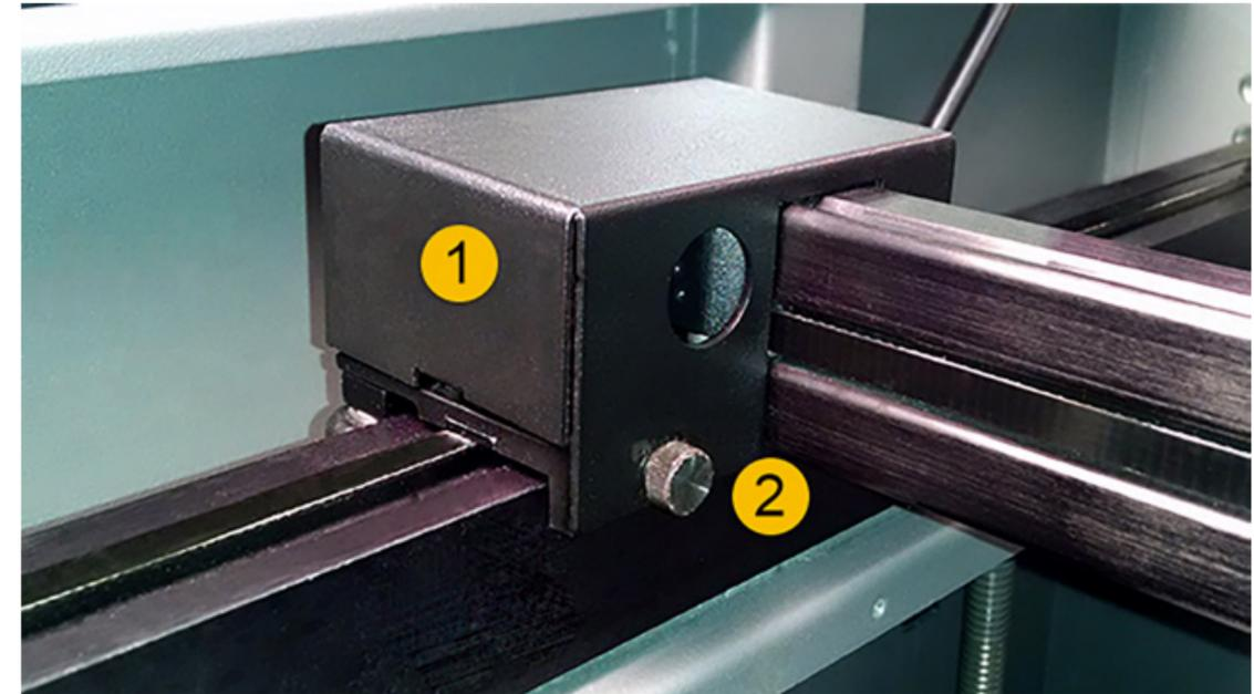
3. Pull the X-axis arm toward the front of the stage until it stops.
