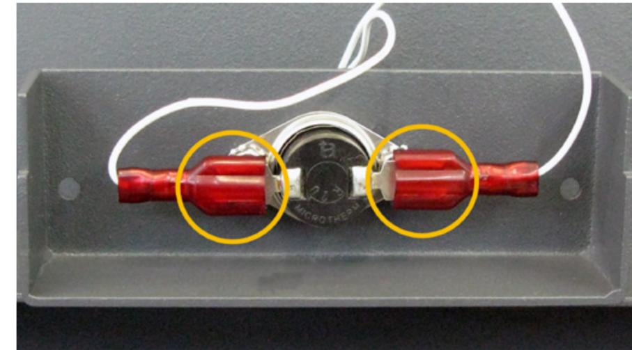
7. Rotate the metal contacts to expose the hex nuts.
