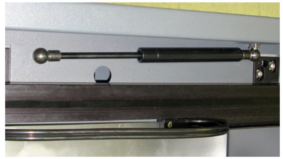
5. Have another person hold the top door and unscrew the 4 screws and washers that hold the top door in place with the hinges. Place the screws and washers in a safe place.
