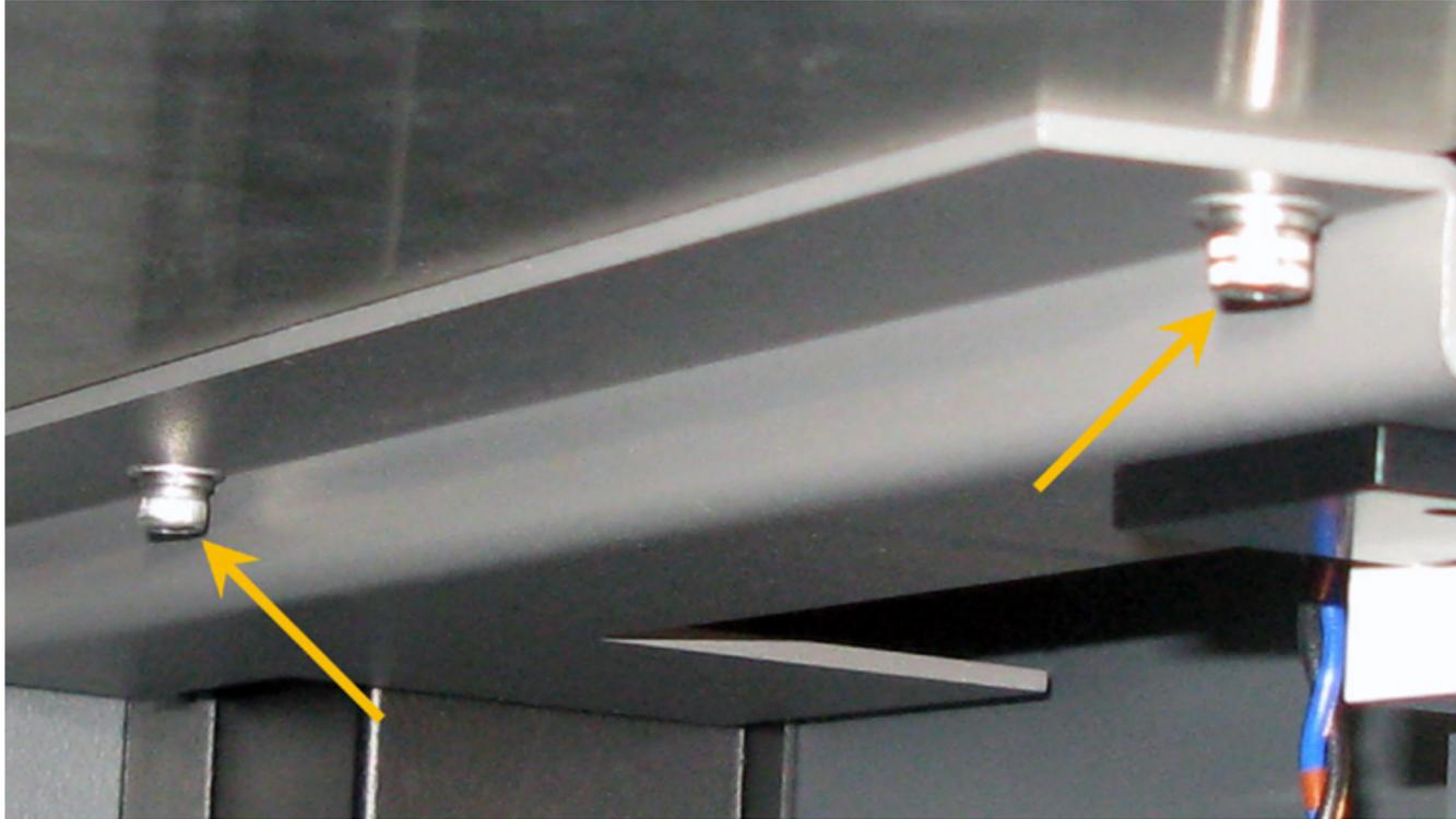
7. Lift the stage out of the system and set it in a safe location being careful not to damage the proximity sensor.
