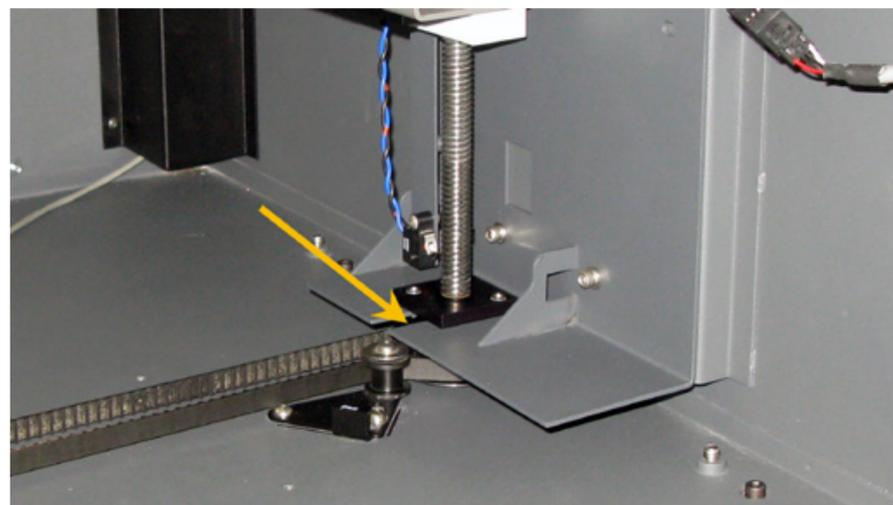
18. Install the Belt Cover with the 6 Buttonhead Screws. Apply fresh white lithium grease to the 3 Lead Screws making sure there is an even coating of grease on the Lead Screws throughout the entire length of travel for the Z-axis Table.
