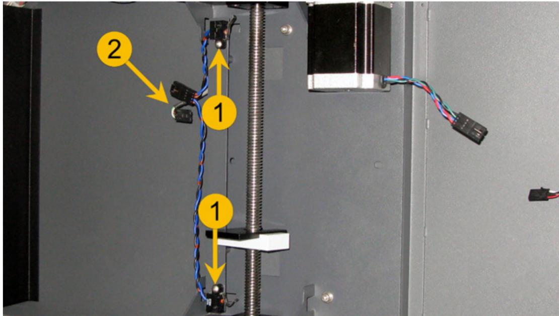
5. Locate near the top switch and disconnect the Z Limit Switch (2) assembly connector by pressing the tab on the connection and pulling gently.
