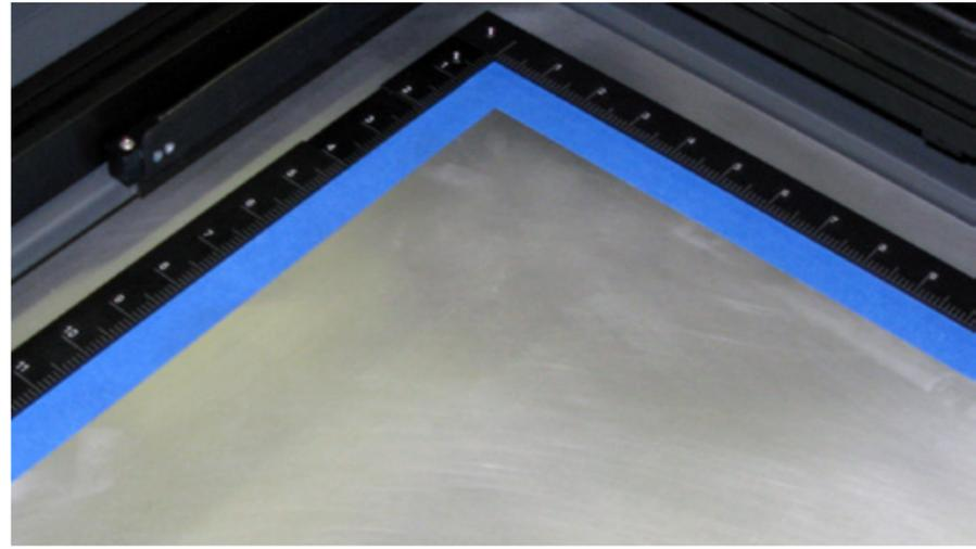
8. Once the rulers are correctly located, reinstall the screws removed in step 1 to secure the rulers to the engraving table.
