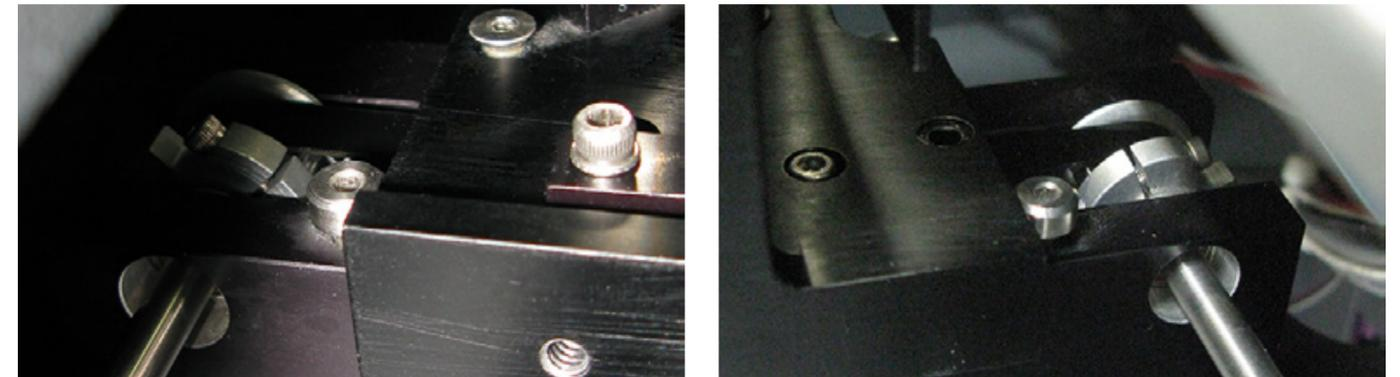
5. If there is a gap between the shoulder screw and the contact point on either the left or right side of the arm, square the arm by making the following Adjustments.
