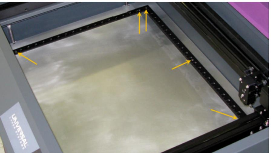
2. Use solvent cleaner to remove any debris left over from the removed rulers.
