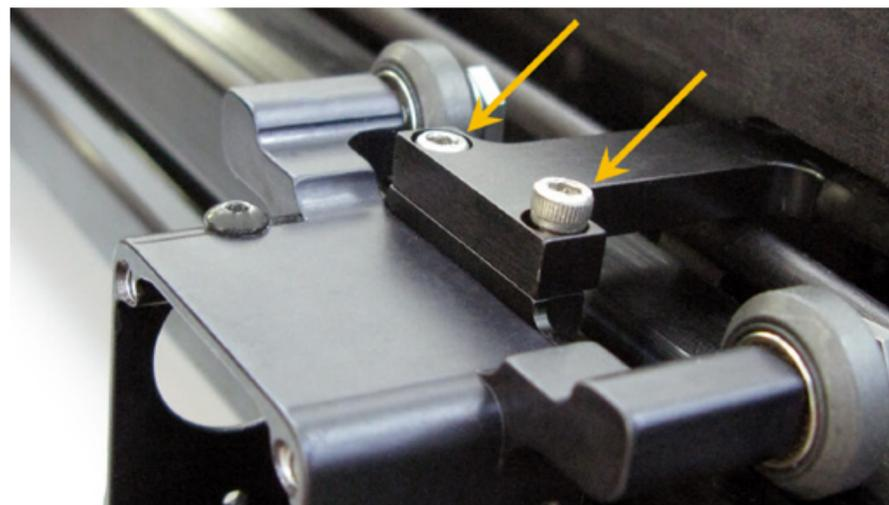
6. Keeping in mind that the bottom bearing in the carriage is spring loaded, grab hold of the Focus Carriage and gently push up, then tilt forward to remove the Focus Carriage from the X-axis Arm.
