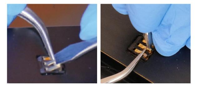
Hold the screwdriver in the other hand with the index finger near the blade. Position the screwdriver so that the flat tip rests between the existing bend and the placement of the closed tweezers.
