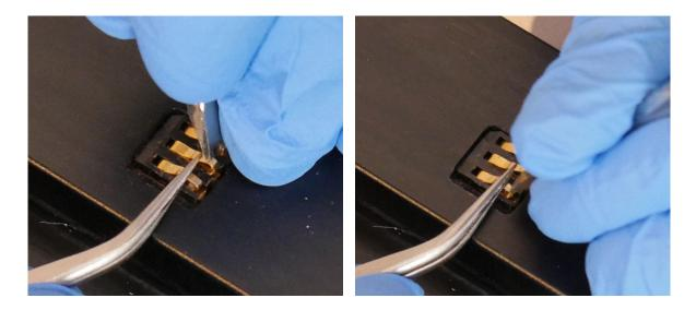
The new bend should be located halfway along the spring finger, approximately 1 mm below the original bend.
