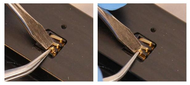
Hold the screwdriver in the other hand with the index finger near the blade. Position the screwdriver so that the flat tip rests between the placement of the closed tweezers and the base of the spring fingers.
