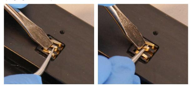
Hold the screwdriver in the other hand with the index finger near the blade. Position the screwdriver so that the flat tip rests between the placement of the closed tweezers and the base of the spring finger.
