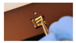
If the adjusted spring fingers are higher than the left spring finger, press down each spring finger at its midpoint with the closed tip of the tweezers.
